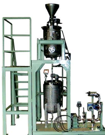
With two tanks and a flow meter.
